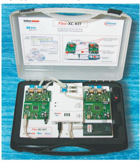
The kit provides an easy access to the FlexRay technology and enables a hassle-free development start.
