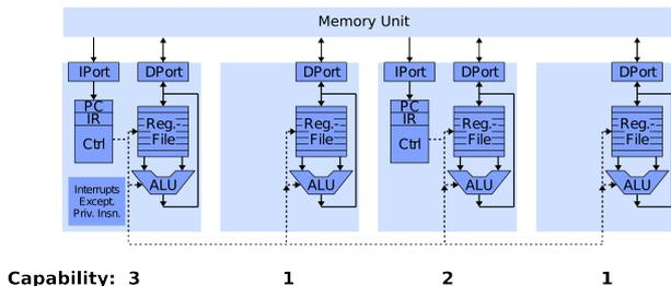
Fig. 4. Example of a *ParaNUT* instantiation with cores of different capabilities
