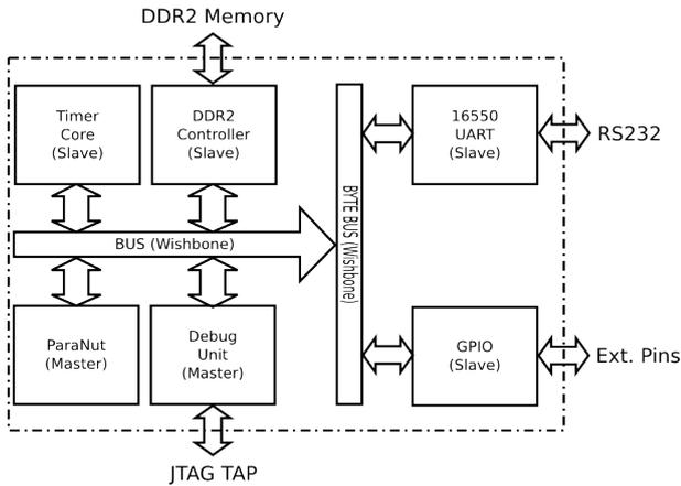
Fig. 6. Block diagram of the evaluation platform system-on-chip
