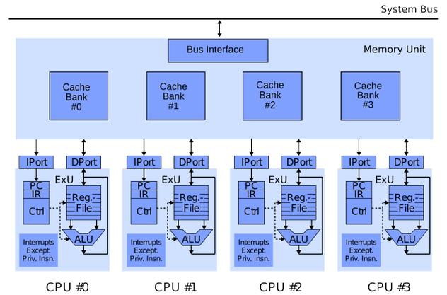
Fig. 1. Block diagram of a *ParaNut* with 4 (full-featured) cores
