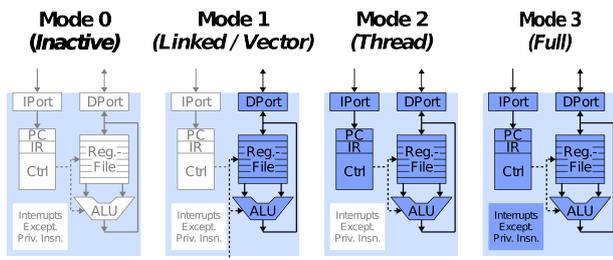
Fig. 3. Modes of a *ParaNUT* core
